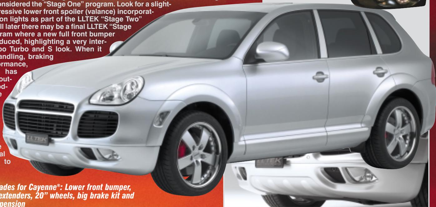
**Styling upgrades for Cayenne®: Lower front bumper, wheel arch extenders, 20" wheels, big brake kit and lowered suspension**
