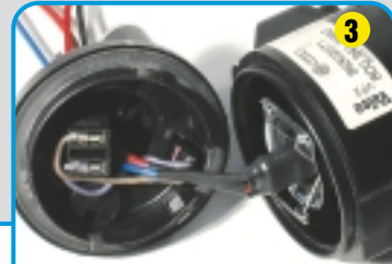
"Click" connect the wires to the Audi bulb socket via direct insertion
