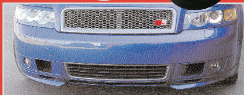
Zender air intake scoops quickly replace the traditional factory setup.
